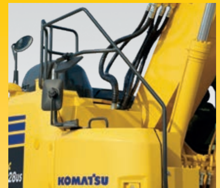
Hand rails and anti-slip plates
