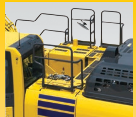
Hand rails and anti-slip plates
