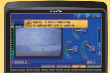
AdBlue® level and refill guidance
