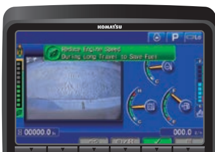
Eco-gauge, Eco guidance and fuel consumption gauge
