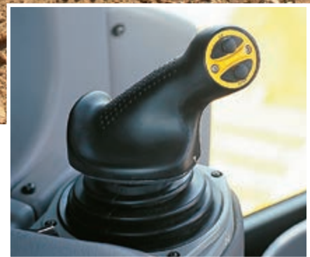
Palm Command Control System (PCCS)
