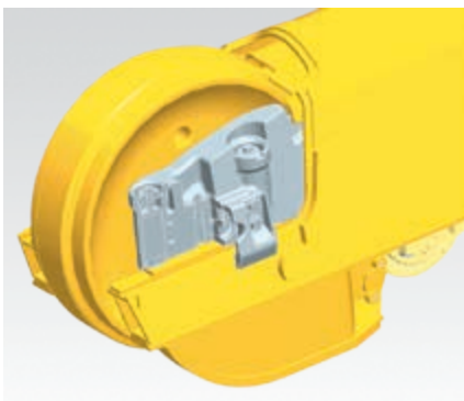
Self-adjusting idler support
