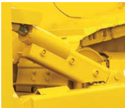
Hydraulic lines are embedded into the structures whenever possible
