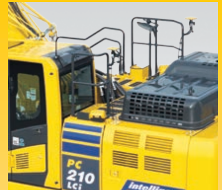
Hand rails and anti-slip plates
