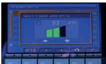
Three pre-set flow selections for Auto Tilt Bucket. Precise finger tip control
