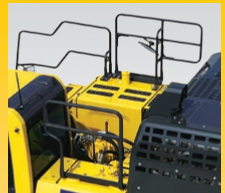
Hand rails and anti-slip plates
