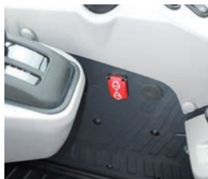
Secondary engine shutdown switch
