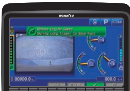
Eco-gauge, Eco guidance and fuel consumption gauge
