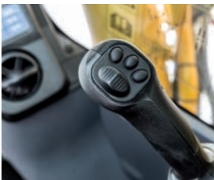
Joysticks with proportional control button for attachments
