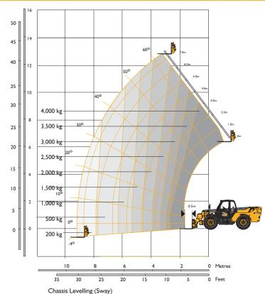
With stabilisers retracted (Sway angle  $\pm 9^{\circ}$ )
