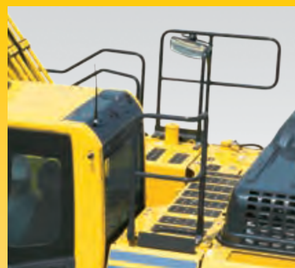
Hand rails and anti-slip plates
