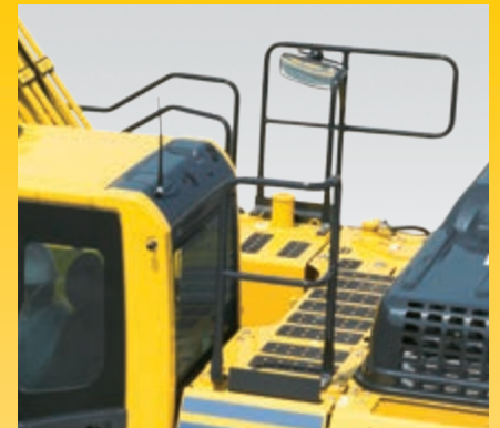
Hand rails and anti-slip plates
