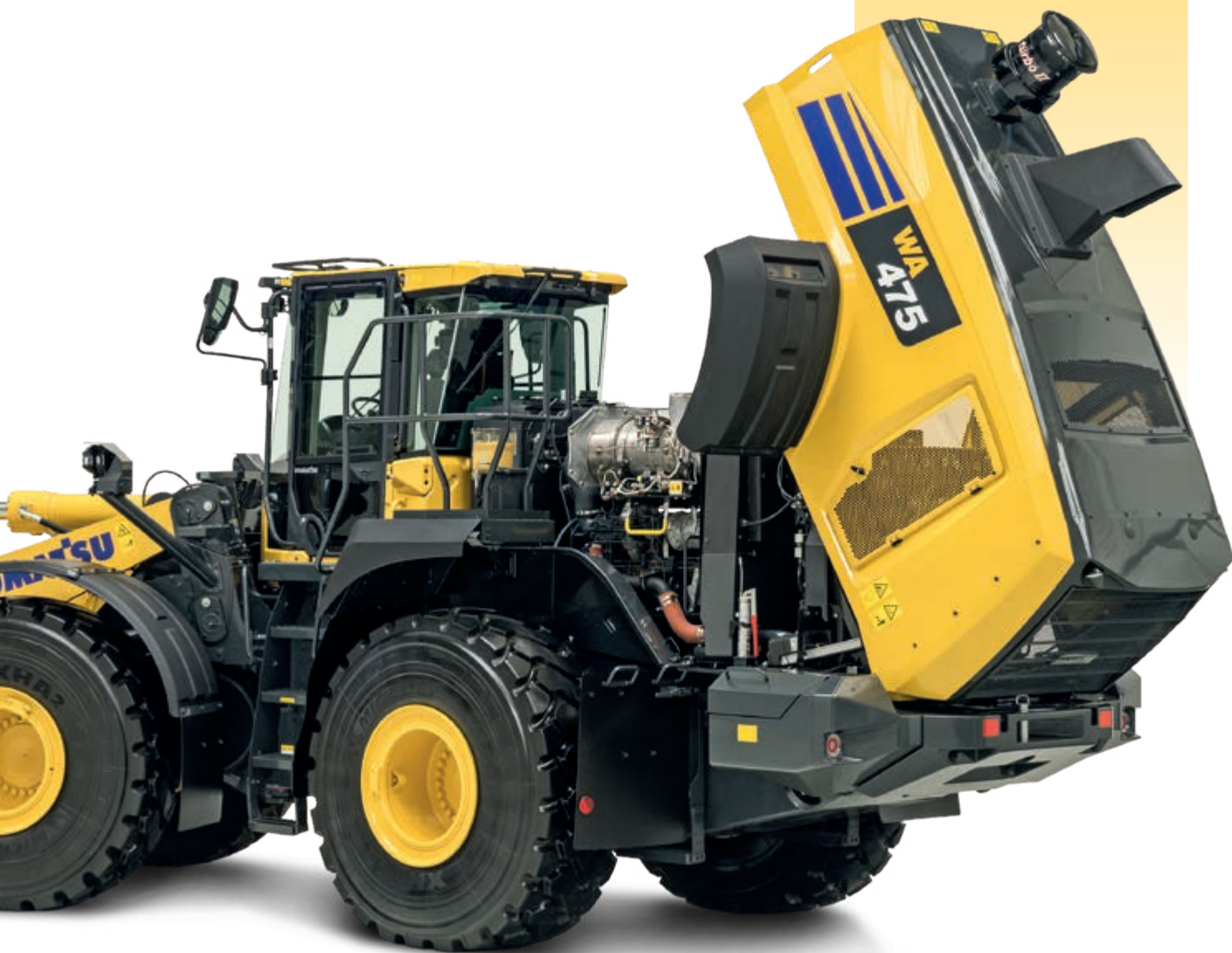
Well located service doors allow convenient and safe access to daily service points
